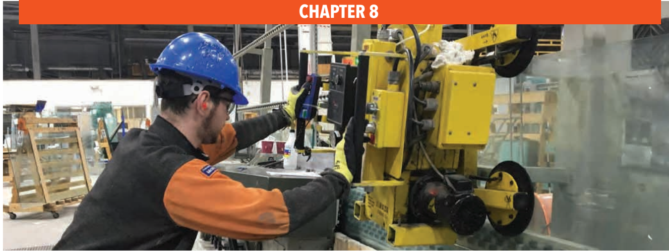
Chris Soden at Syracuse Glass Company uses a glass lifter to place sheets of glass on a conveyor for edge polishing.
